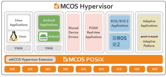
\* MK: Microkernel, VMM: Virtual Machine Monitor
